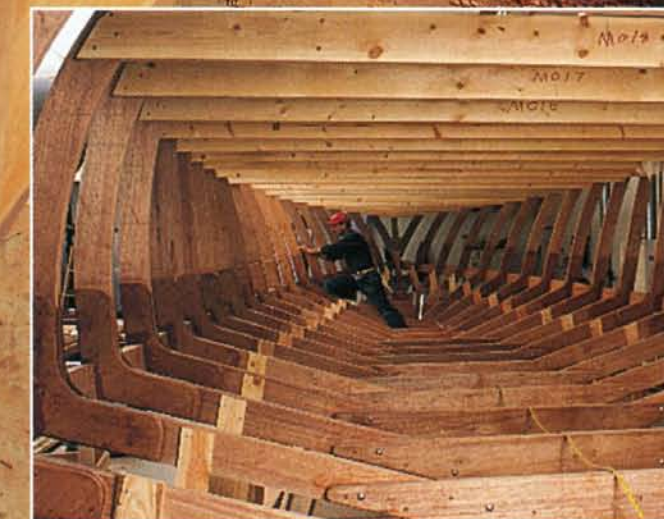
A new Mays-Craft takes shape in the woodworking shop. The same boat (inset) at an earlier stage, looking forward from the transom. Frames, gussets, and floor timbers are all mahogany.
